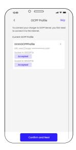
If the desired third-party OCPP is not shown in the existing OCPP profile list, you can add a new profile through the Install APP (you will need to input the Profile Name and OCPP URL). After adding it, you can proceed to connect. If the connection is rejected, please contact Raedian to confirm whether the profile has been integrated.
