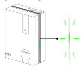
Tap the RFID card above the card reader area until you hear a beep. The charging session will start automatically and the charger's LED will turn cyan with a falling drop effect.
